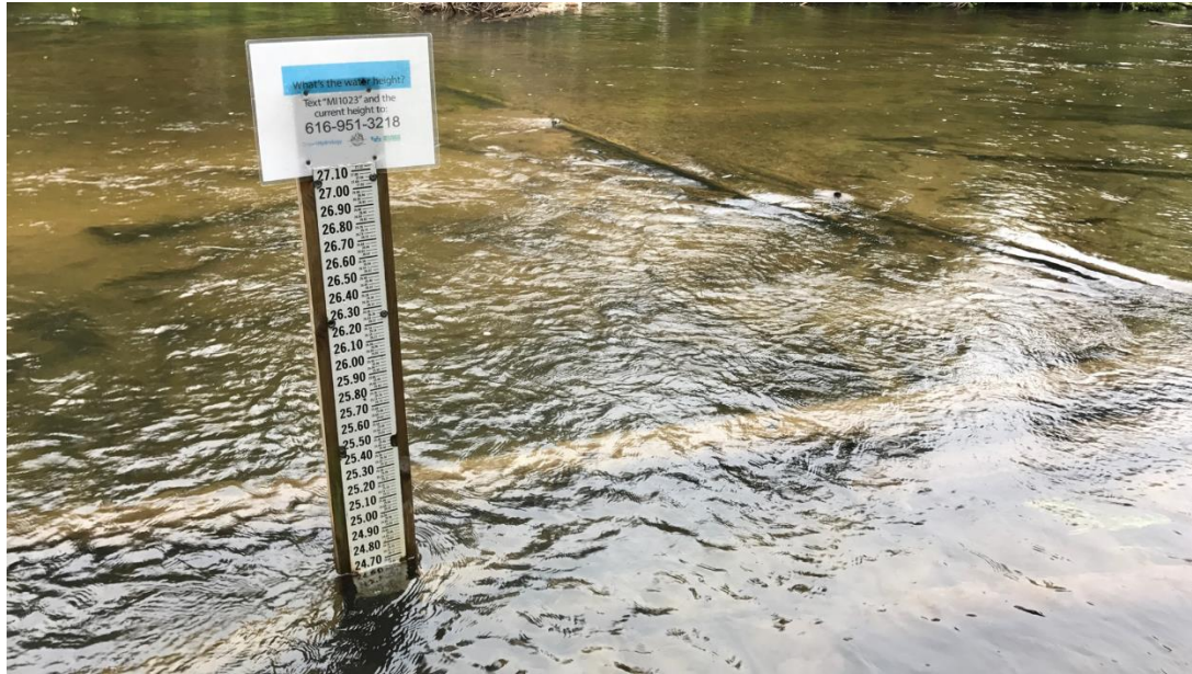
Figure 1. Stream-flow (water height) gauge.
