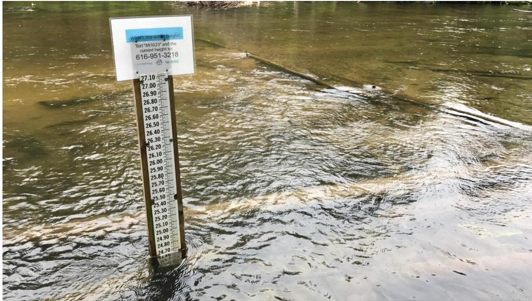
Figure 1. Stream-flow (water height) gauge.
